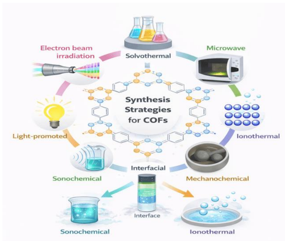
Figure 2. Overview of synthesis strategies for covalent organic frameworks (COFs). Figure 2. Overview of synthesis strategies for covalent organic frameworks (COFs). Schematic representation summarizing the principal synthetic routes employed for the preparation of two- and three-dimensional COFs. The strategies are broadly classified based on reaction environment and energy input, encompassing solvent-mediated thermal methods, energy-assisted approaches, and interface- or mechanically driven processes. These diverse pathways enable controlled framework formation under a wide range of experimental conditions. Adapted from [22].
