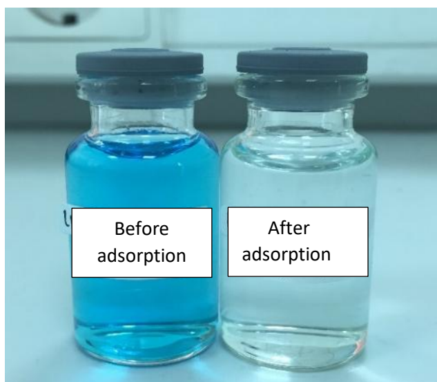
Figure 6. Methylene blue waste before and after adsorption.
