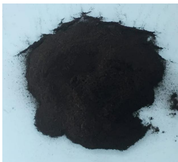
Figure 1. Powder tea waste – \text{Fe}_3\text{O}_4 adsorbent.
